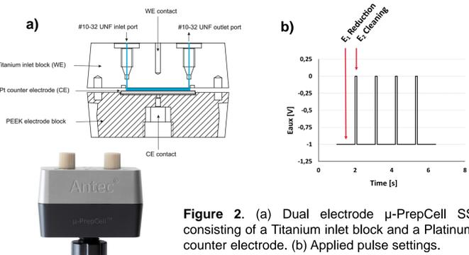
**Figure 2.** (a) Dual electrode  $\mu$ -PrepCell SS consisting of a Titanium inlet block and a Platinum counter electrode. (b) Applied pulse settings.
