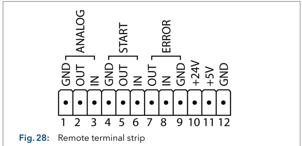
**Fig. 28:** Remote terminal strip
