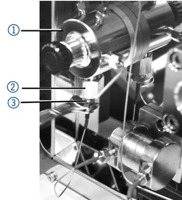
**Fig.39:** Loosen the capillary
