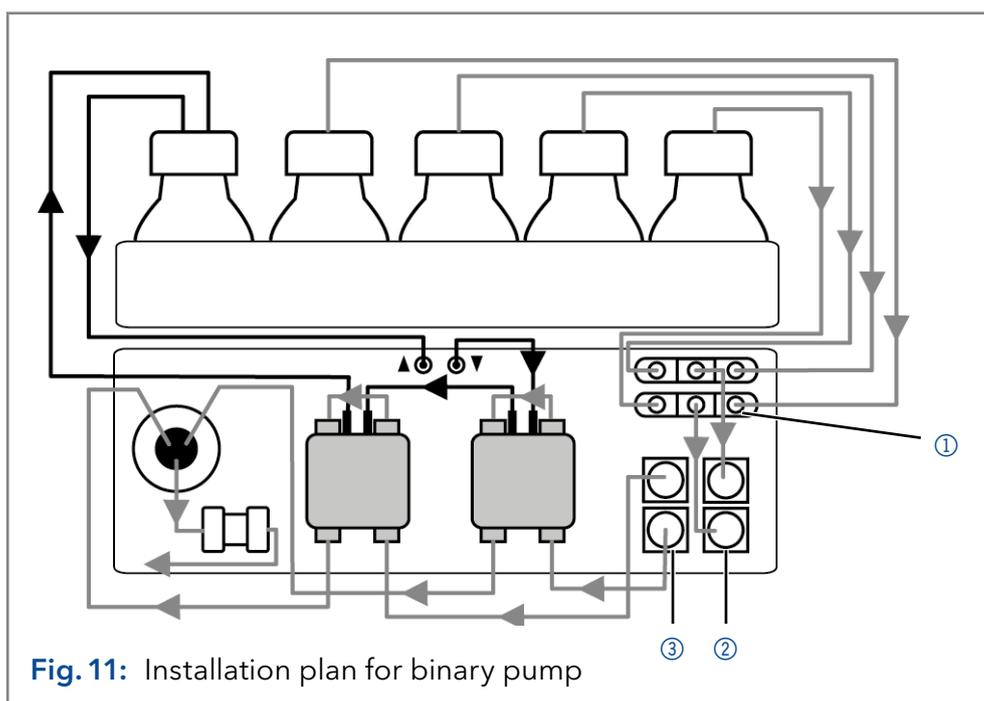
**Fig. 11:** Installation plan for binary pump**Piston backflushing**
