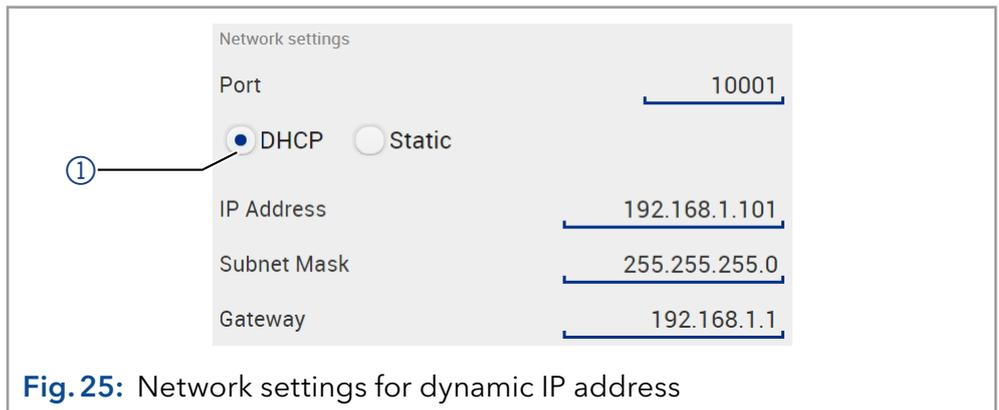
**Fig. 25:** Network settings for dynamic IP address
