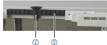
**Fig. 18:** Funnel and capillary guide
