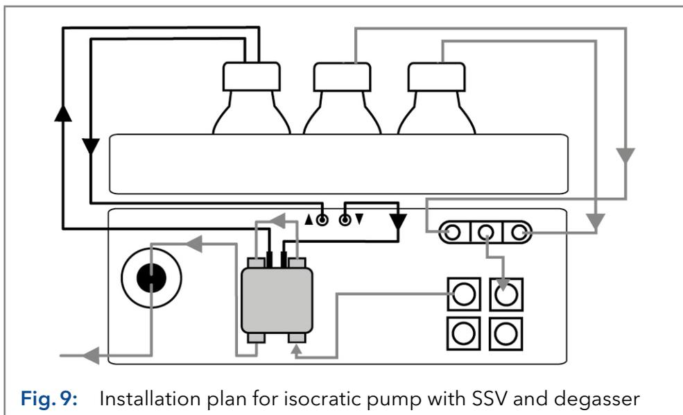
**Piston backflushing** The flushing solution is re-used. Since the flow path is circular, only one bottle is used for the flushing solution.
