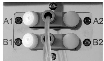
**Fig. 12:** Solvent selection valve with cap fitting
