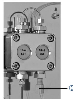
**Fig. 10:** Solvent line on pump head**Next step**
