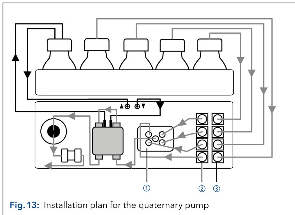
**Fig. 13:** Installation plan for the quaternary pump
