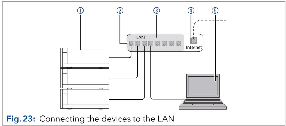
**Fig. 23:** Connecting the devices to the LAN
