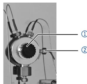
**Fig.31:** Venting screw of the pressure sensor
