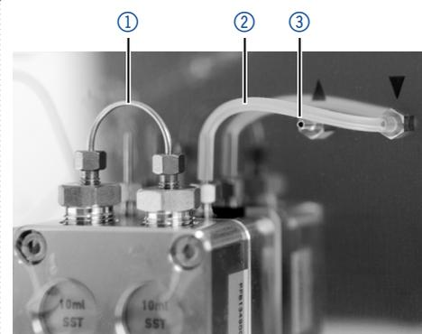
**Fig. 17:** Connecting piston backflushing
