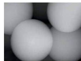
SEM image of 5 µm SweetSep particles
