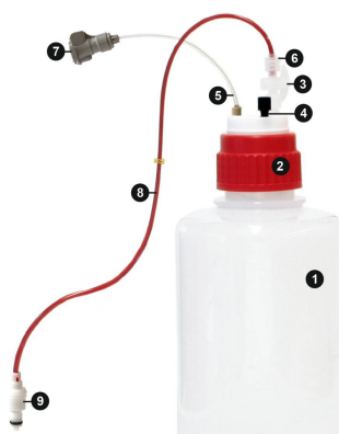
Figure 2. The PPCO bottle assembly includes: (1) PPCO bottle, (2) B53 cap with three \frac{1}{8} -28 ports, (3) 2-way stopcock, (4) \frac{1}{8} -28 PP plug, (5) mobile phase line, (6) \frac{1}{8} " OD tubing with Luer connector, (7) quick connector for mobile phase line, (8) inert gas supply line, and (9) quick connector for inert gas line. Each bottle features quick, auto-sealing connectors that prevent spills of high-pH eluents, improving laboratory safety.
