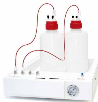
Figure 1. The ET 210 has four gas outlets for up to four mobile-phase bottles, each kept under an inert gas atmosphere (blanketing), reducing costs by using \text{N}_2 instead of He. Safety valves regulate inlet and outlet pressure, preventing bottle over-pressure and ensuring operator safety.
