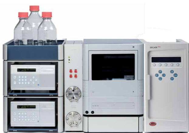
Figure 1: ALEXYS Aminoglycosides Analyzer for Spectinomycin.
