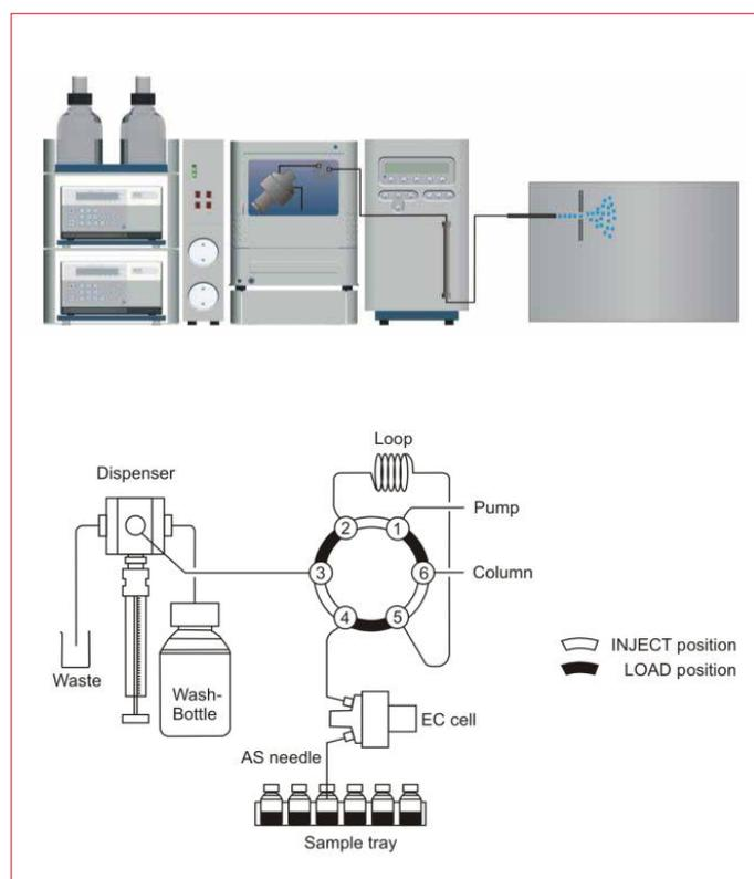
**Figure 3:** Top: ROXY™ EC/LC System including ReactorCell™ integrated in the AS110 autosampler flow path. Bottom: Detailed lay-out of autosampler flow path with 6-port injection valve and ReactorCell™
