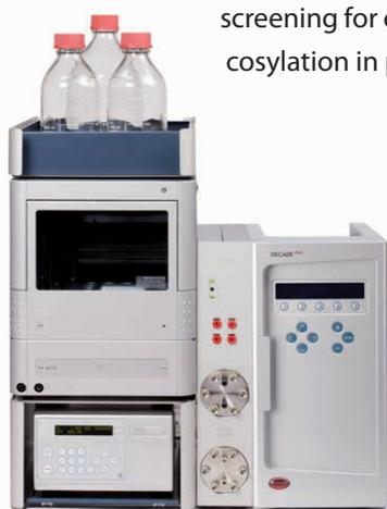
**Figure 1:** ALEXYS Carbohydrate analyzer for isocratic HPAEC (mono- and disaccharides).
