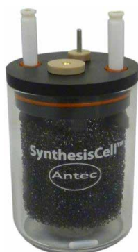
Figure 1: SynthesisCell™ with Reticulated Glassy Carbon (RGC) working electrode (WE), a Pd/H 2 reference electrode (HyREF), and a Pt auxiliary electrode (AUX).
