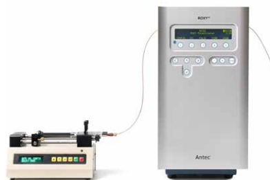
Figure 10: ROXY™ EC System consisting of ROXY Potentiostat, dual syringe pump and ReactorCell.
