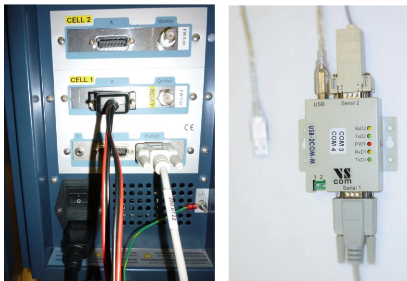
Fig. 3. Back panel of a ROXY Potentiostat (left) and VScom RS232-USB converter. Converter is connected to computer using an USB port.
