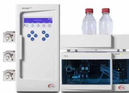
ALEXYS Neurotransmitter Analyzer for high throughput. Three valves and one pump with a flow splitter are used for three HPLC channels running in parallel.
