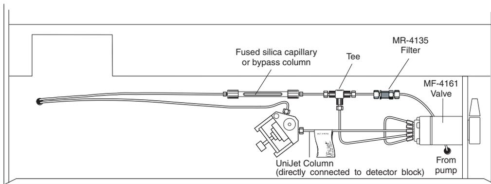
Figure 8. BAS 200B using a flow splitter
