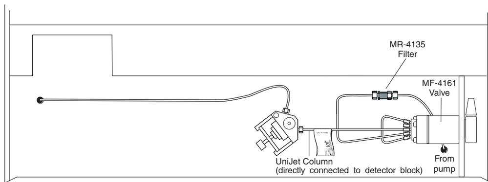
Figure 9. BAS 200B – direct connection to pump
