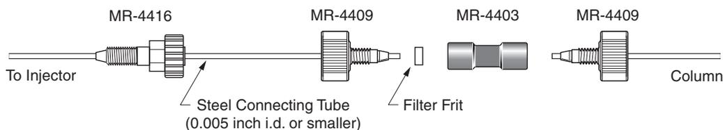
Figure 6. Installation of MF-8952 microbore in-line filter kit. This filter has a very low dead volume and is the only filter recommended between the injector and column inlet.
