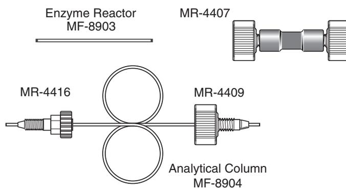
*Figure 2. UniJet microbore ACh/Ch analytical column and IMER.*
