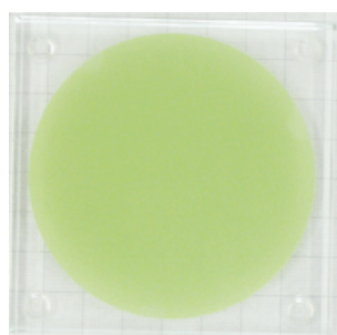
Fig. 11. Green polishing disc for FS column outlet.
