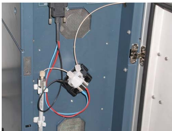
Fig. 9. Installation of the Sencell in a DECADE II.
