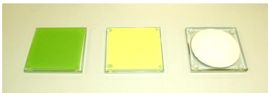
Figure 1a. 30 um flattening plate (green), 12 um flattening plate (yellow) and polishing disc.
