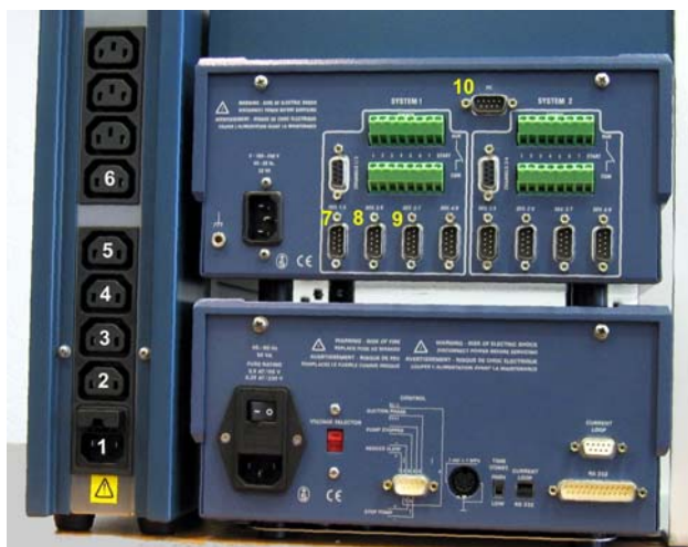
Fig. 9. Back view of the OR 100 with LC 100 pump and AC 100. Connectors 1 – 10 are numbered for reference.
