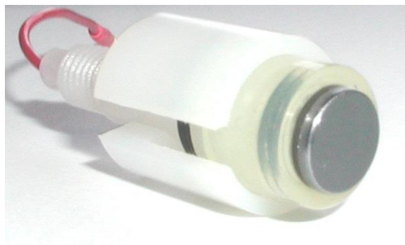
Fig. 9. Working electrode assembly with Magic Diamond electrode .
