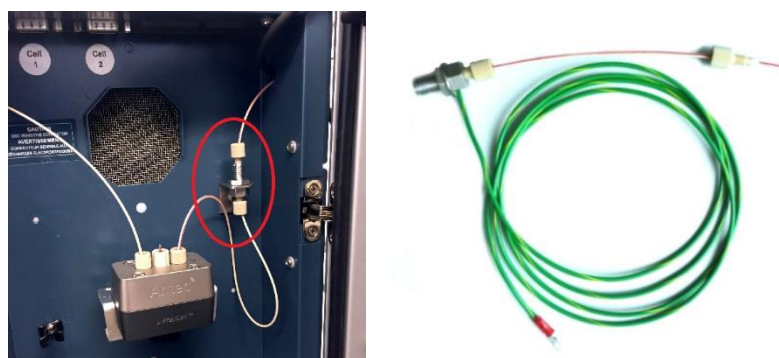
Fig. 5. The grounding kit inside the ROXY (left) or for external use (right).
