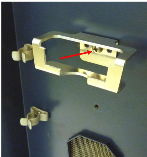
*Figure 6.  $\mu$ -PrepCell holder mounted on the center position in the ROXY potentiostat oven compartment.*
