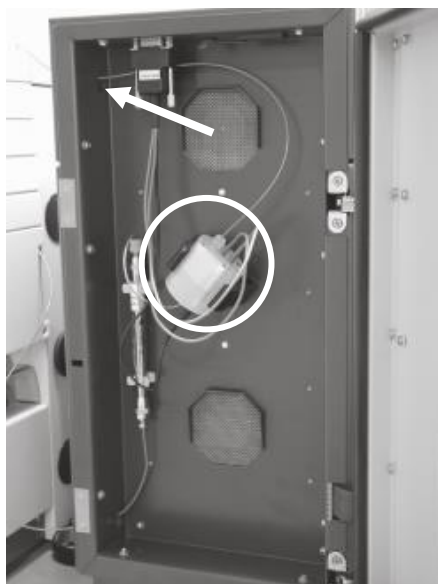
Fig. 1. Take out the flow cell and place temperature sensor within the area indicated with the white circle. Insert the temperature probe via the tubing hole (arrow) and close the door.
