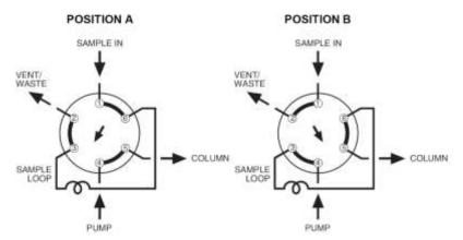
Fig. 61. Example of the valve flow path of a 6-port valve.
