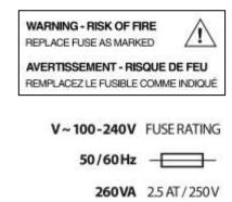
Replace blown fuses with fuses of proper type and rating as indicated on the rear panel and as listed in the list of accessories and spares (appendix D). The fuse holder is integrated in the mains connector. Ensure that the instrument is never put in operation with fuses of a different type. This could cause fire.
