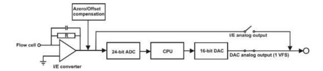
Fig. 64. Top: CONFIG screen. Bottom: DECADE Elite signal processing from electrochemical flow cell to output. R is a selectable I/E resistor of 100M, 10M, 1M, 100K, 10K or 1K in the I/E converter circuit.
