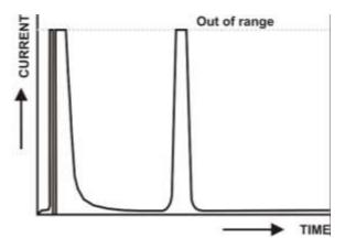
Fig. 66. Example of a chromatogram were the cell current exceeds the maximum current level and the signal is 'out of range'.
