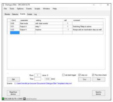
Fig. 69. Dialogue Elite Event table window with an example of programming timed events for output A (in this case Relay 1).
