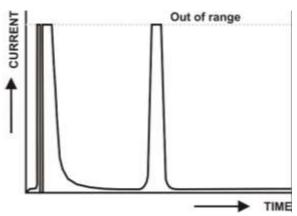
Fig. 72. Example of a chromatogram were the cell current exceeds the maximum current level and the signal is 'out of range'.
