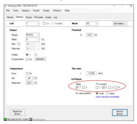
Fig. 67. Dialogue Elite Detector tab with I/O status and control buttons.
