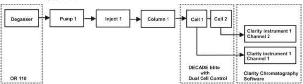
Fig. 16. Typical configuration for serial mode detection. Cell 1 is a FlexCell, cell 2 is a SenCell for detection. Channel 1 and 2 use the same time base of system 1.
