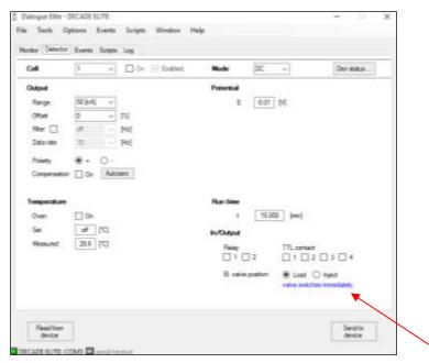
Fig. 59. DECADE Elite detector window with Valve control.
