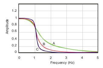
Fig. 37. An amplitude response plot of a low pass filter with a cut-off frequency of 1 Hz. It is a 2 (A), 4 (B) and 8 (C) pole Bessel filter.
