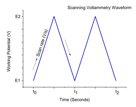
Fig. 46. Scanning voltammetry potential waveform.
