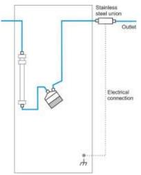
Fig. 71. Left: DECADE Elite rear panel grounding stud. Right: example of shielding the flow cell by grounding the solvent outlet tubing.
