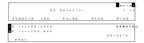
Fig. 19. DECADE Elite main menu (top) with active cell indicator in top right corner. Multi-STAT screen showing cell 1 (DC mode) and cell 2 (PULSE mode).
