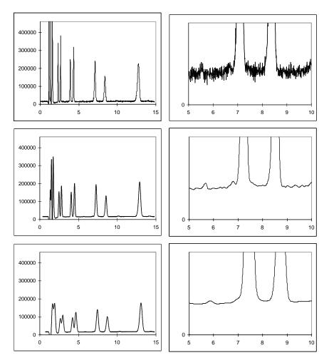
Fig. 39. From top to bottom filter setting of 0.5, 0.02 and 0.002 Hz. Narrow peaks in front of the chromatogram are deformed at 0.005 Hz, whereas wider peaks show hardly any deformation (see peak at t~ 13 min). Attenuation of noise is shown in the close up on the right.
