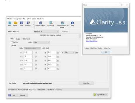
Fig. 10. DECADE Elite method window in Clarity. On the main tab the main measurement conditions can be set/controlled (measurement mode & potential settings).
