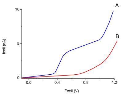
Fig. 47. Scanning voltammetry of 1.0 µmol/L norepinephrine (A) at a glassy carbon working electrode, at a scan speed of 10 mV/s. Scan (B) is the blank solvent.
