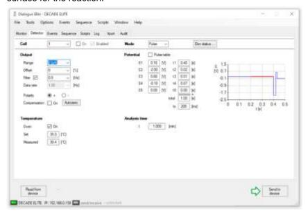
Fig. 25. Pulse mode method settings window in Dialogue Elite. The potential waveform settings are shown on the right side.
