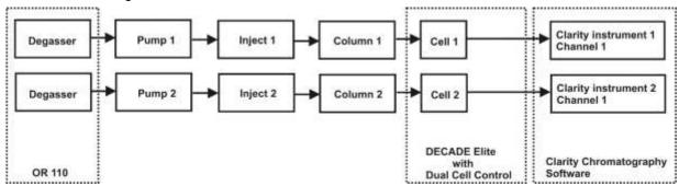
Fig. 17. Typical configuration for parallel mode detection. Two independent HPLC systems with dual channel support from OR 110, DECADE Elite and Clarity software.
