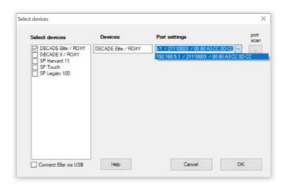
When a DECADE Elite detector is available it is automatically detected and the IP address is shown in the port settings box. If not press port scan or type in the default IP address 192.168.5.1.
