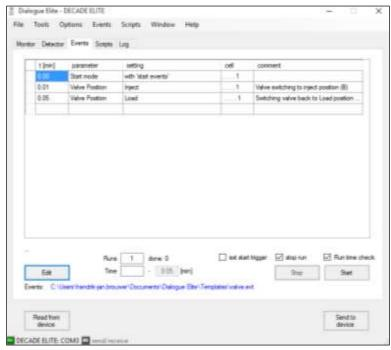
Fig. 63. Dialogue Elite Events tab with an example of two programmed events switching the valve to Inject (t = 0.01 min) and back to Load (t = 0.05 min).
