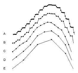
Fig. 43. A detailed part of a chromatogram acquired at different data frequencies. The data rate is (A) 5x, (B) 2.5x, (C) 1.2x, (D) 0.6x and (E) 0.3x the frequency of the pulse. C is 1 Hz data rate.
