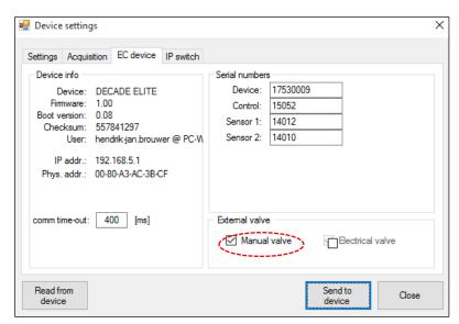
Fig. 60. Dialogue Elite EC device settings, manual valve check box.
