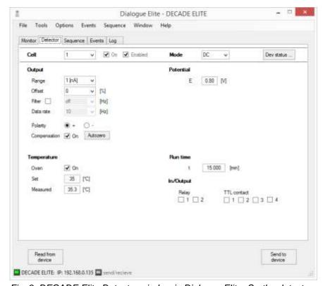
Fig. 8. DECADE Elite Detector window in Dialogue Elite. On the detector tab the main measurement conditions can be set/controlled (measurement mode & potential settings)
