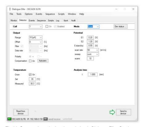
Fig. 29. Scan mode method settings window in Dialogue Elite. Continuous scan (10 scans) between 0.20 and 1.20V with a scan rate of 50 mV/s.
