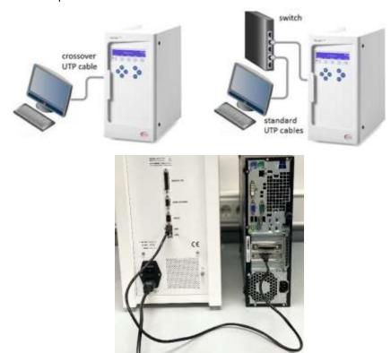
Fig. 3. Example of LAN connection between PC and DECADE Elite. A direct connection requires the special crossover UTP cable delivered in the detector ship kit. With a Ethernet switch any regular UTP cable can be used.
