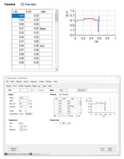
Fig. 27. The new pulse mode 2 with freely programmable t,E table. In red the sampling of data for acquisition.
