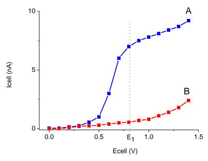
Fig. 45. Hydrodynamic voltammogram of norepinephrine (A) at a glassy carbon working electrode, and the current of the baseline (B). At  $E_1$  the electrochemical signal becomes diffusion limited.
