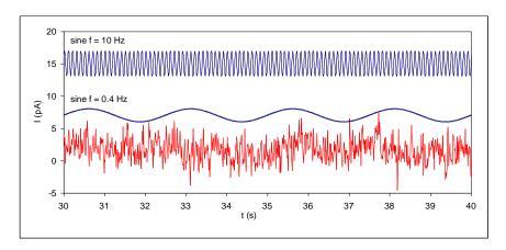
Fig. 35. Typical random noise in chromatography (lower trace). Both frequencies (0.4 and 10 Hz) can be recognized amongst others.
