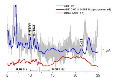
Fig. 40. Analysis of 20 pmol/L 5-hydroxytryptophan, 5-HIAA and 5-HT using ADF for improving detection limits.
