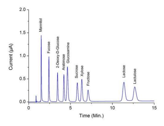
Fig. 41. Carbohydrate analysis in the pulse mode.
