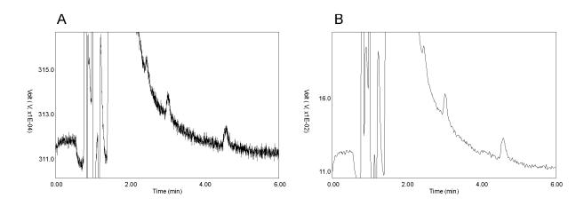
Fig. 21. Signal to noise ratio is improved using a filter (A vs. B).
