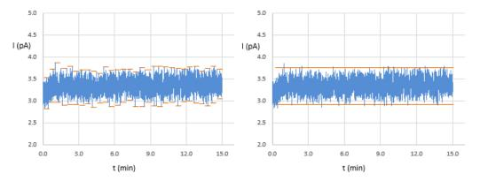
Fig. 74.Baseline noise measurement from 30 segments (left) and an estimate (right). The noise in both cases is 0.8 pA.
