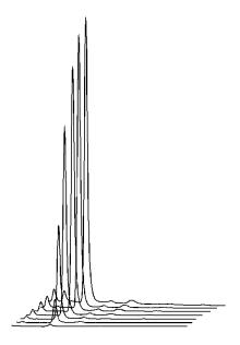
Fig. 50. Construction of a hydrodynamic voltammogram for norepinephrine. Chromatograms are obtained at cell potentials ranging from 1.0 V (back) to 0.4 V (front), with 100 mV steps.
