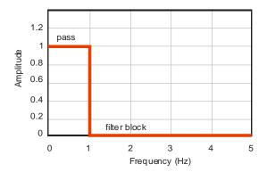
Fig. 36. Amplitude response plot of an ideal low pass filter with a cut-off frequency of 1 Hz.
