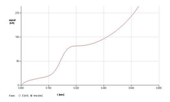
Fig. 55. Scan (cycle: half) of a 20  $\mu$ M Serotonin in mobile phase at a glassy carbon working electrode. Scan speed 20 mV/s.
