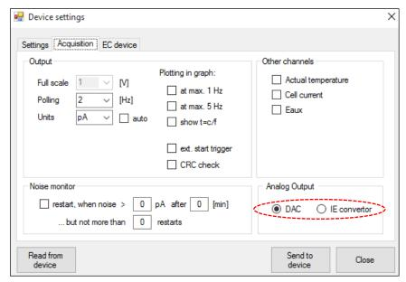
Fig. 65. Dialogue Elite Acquisition tab analog Output setting.
