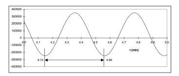
Fig. 31. Sine of Fig. 30. A full period is 0.41 min (25 s) which corresponds to a frequency of 1/25 = 0.04 Hz.
