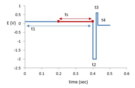
Fig. 42. Potential steps in pulsed amperometric detection. During t1 the detection potential is applied, detection occurs during ts. Steps t2, t3 and t4 are for regenerating the electrode. This process repeats itself continuously as soon as the cell is on.
