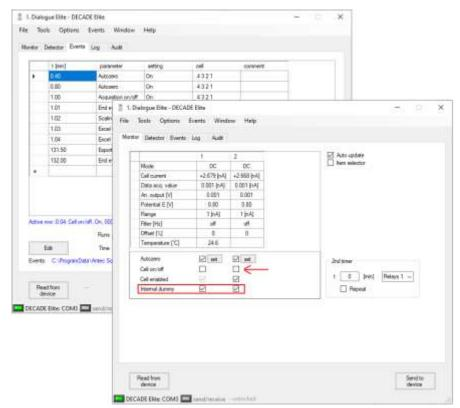
Fig. 75. After starting the "Dummy cell noise test", the internal dummy cell must be checked. Note that the (external) cell is off.
