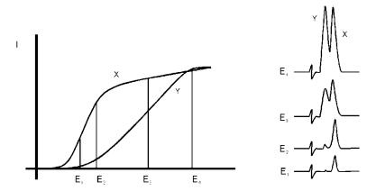
Fig. 48. Selectivity in LC-EC of compound X and Y is optimised by choosing the working potential with the largest difference in peak height.
