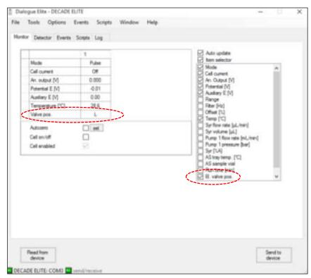
Fig. 62. Dialogue Elite Monitor tab with valve status (position) displayed.
