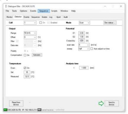
Fig. 52. Programming a scan in the Elite Dialogue software, half sweep.
