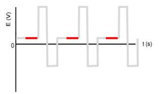
Fig. 24. Pulse mode example: Plot of a three-step potential waveform (grey curve) versus time. Red part: time during which the current signal is measured.
