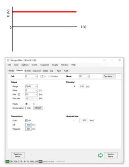
Fig. 23. Top: Plot of cell potential versus time. Bottom: DC mode method settings window in Dialogue Elite. The potential (top right) can be set between -2.5 and +2.5 Volt.
