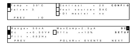
Fig. 20. Selection of parameters in the 'DC SETUP' screen. Temperature is set in CONFIG menu.
