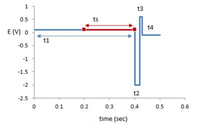
Fig. 26. Potential steps in pulse mode. During t1 the measurement potential is applied, the actual current measurement occurs during ts. Steps t2, t3 and t4 are for regenerating the electrode. This process repeats itself continuously as soon as the cell is on.
