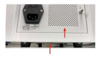
Fig. 2. Location of ventilation holes in the DECADE Elite (bottom & rear).
