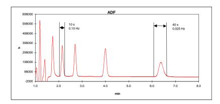
Fig. 34. Typical chromatogram with peak widths between 10 – 100 s.
