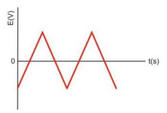
Fig. 28. Scan mode example: plot of cell potential versus time in scan mode (two full scans).
