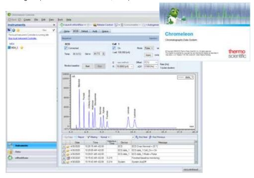
Fig. 11. Chromeleon console showing a ECD e-panel with method settings and acquisition window.
