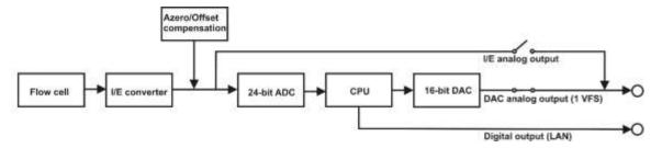
Fig. 15. DECADE Elite signal processing from electrochemical flow cell to output.
