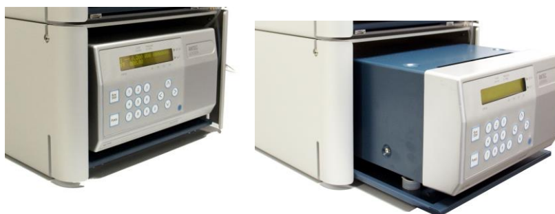
Fig. 25. Accessing the LC 110S pump.
