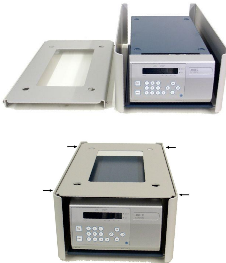
Fig. 23. Top: PR 110 with stacker removed to insert pump. Bottom: PR 110 with stacker assembled (arrows marking the allen screws to fix stacker on frame).
