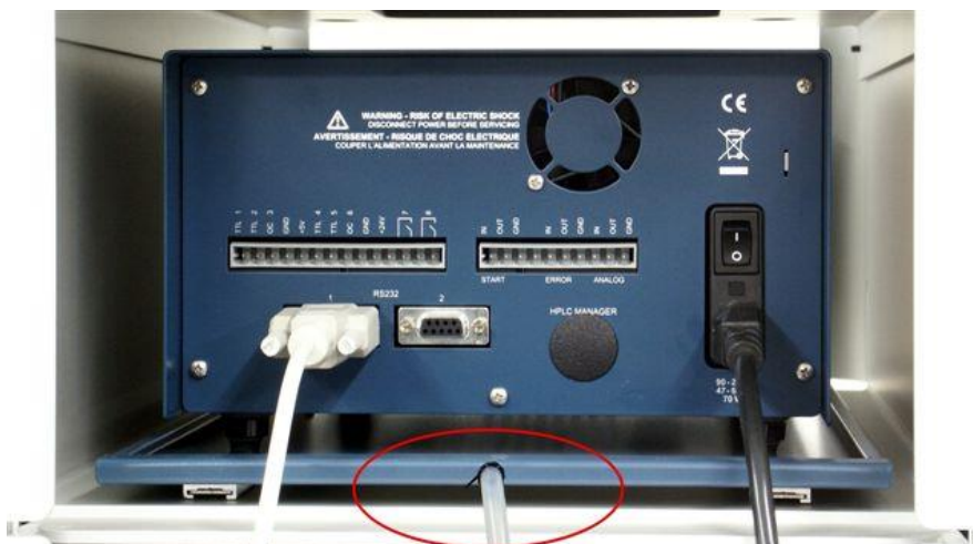
Fig. 24. Rear view of LC 110S in the PR 110 pump rack. The drain is encircled in red.
