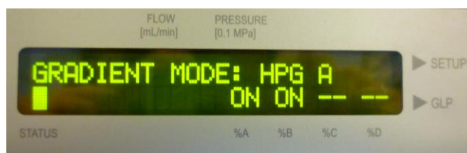
Fig. 17. Pump display when gradient mode for 2 pumps (HPG A and HPG B) is properly set. The first pump was configured as HPG A and both channels indicating %A and %B are ON.
