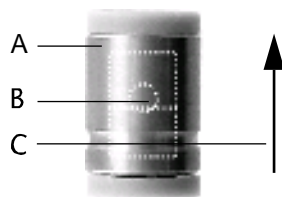
Fig. 40. Functional principle and flow direction of the check valve. A. Check valve, B. Ruby closing ball C. Flow direction. Note the ribbon on the side of the check valve cartridge, this indicates the direction of flow.
