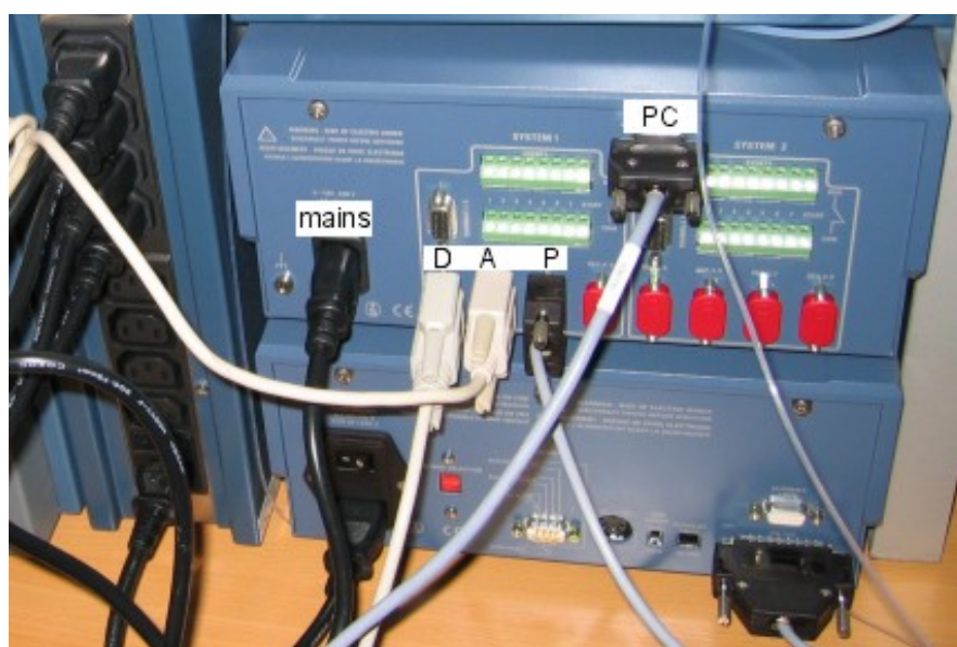
Fig. 3. Rear panel connectors AC 100. D - A - P refers to d etector, a uto sampler and p ump. 'PC' is connection with computer; 'mains' is connected to OR 100.
