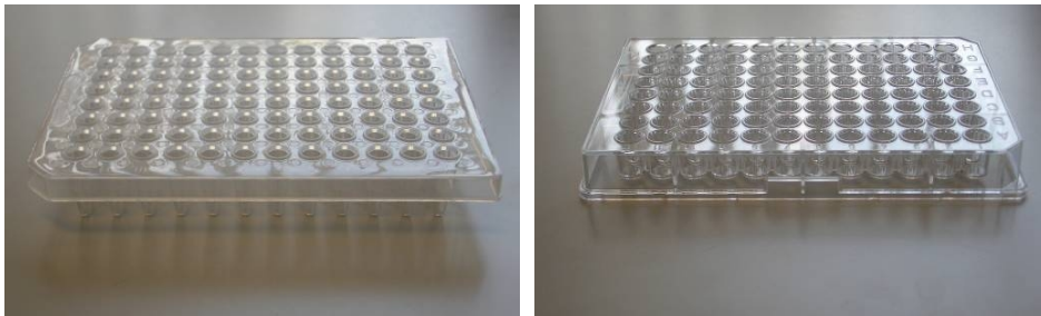
Fig. 2 Left: transparent 96-positions plate (reordering info: Greiner bio-one, pn. 652280), and right: 96-positions flat bottom plate holder (reordering info: Greiner bio-one, pn. 655101).
