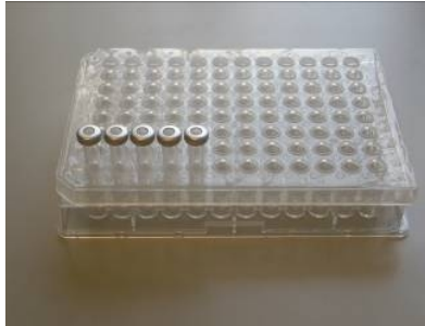
Fig. 1 Assembly of 96- positions base plate and PCR plate with 5 inserted fraction collector vials.
