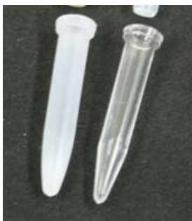
Fig. 3. Picture of two slightly different fraction collector vials. The subtly slimmer type on the right side will fit in the 96 positions tray of the autosampler. For the slightly wider type on the left, adapters are necessary, which fit in the 48 positions tray.
