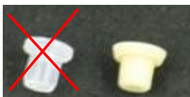
Fig. 4. Typical fraction collector caps, recloseable. Do not use the hard plastic type on the left, as this may damage the needle of the autosampler. The soft rubber type on the right can be used.
