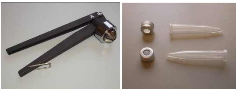
Fig. 3. Crimper tool, caps and vials shipped with each ALEXYS neurotransmitter analyzer.
