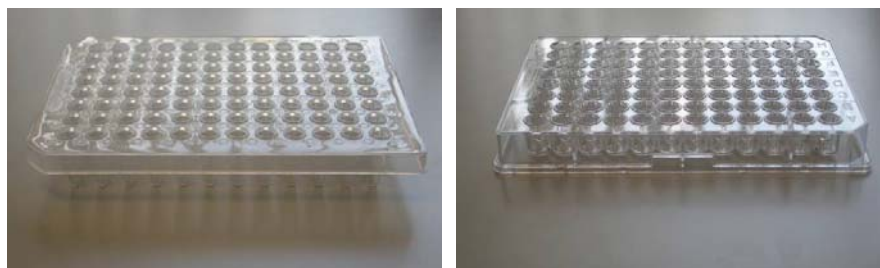
Fig. 2 Left: transparent 96 positions PCR plate (re-ordering info: Greiner bio-one, pn. 652280), and right: 96 position flat bottom plate holder (re-ordering info: Greiner bio-one, pn. 655101).
