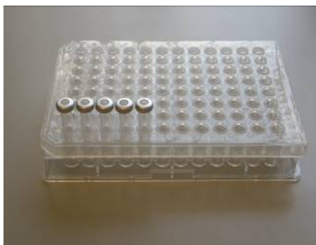
Fig. 1 Assembly of 96-positions PCR plate with 5 fraction collector vials.
