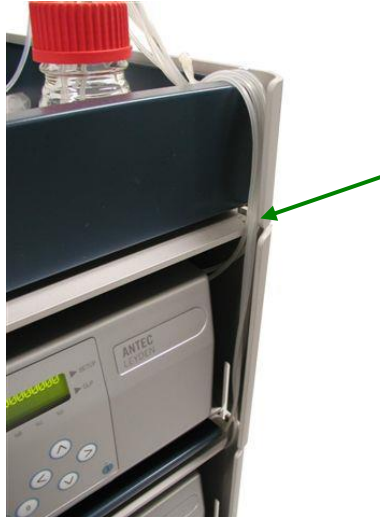
Figure 11. Lead the piston wash up to the solvent tray trough the rim of the pump racks (green arrow).
