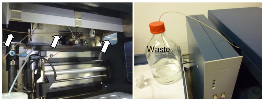
Figure 14. Picture of the autosampler with the waste tubing arranged through the valve compartment and into the waste bottle.
