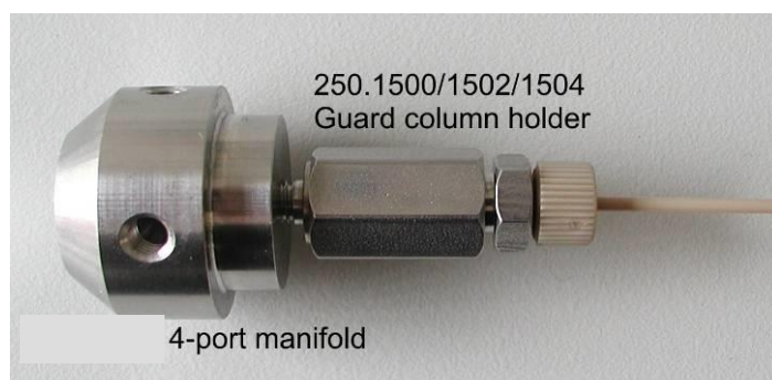
Figure 18. 4-port manifold with guard column holder. Notice that the manifold supplied with the system is already prefixed on a mounting bracket
