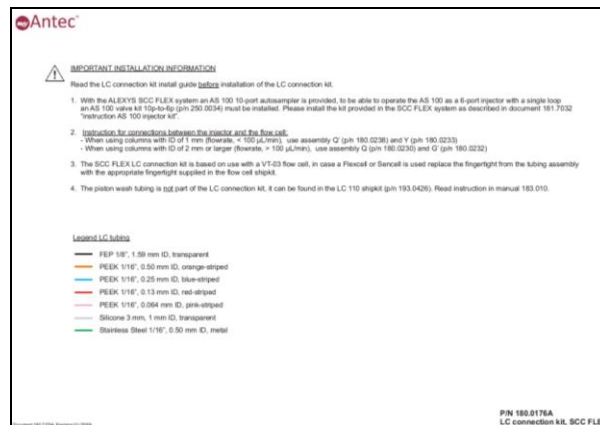
Figure 4. Example of back side of an LC connections schematic drawing with additional application specific info (see text).
