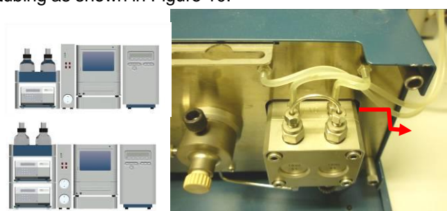
Figure 10. The piston wash inlet and outlet tubing is manoeuvred behind the short interconnecting tubing to secure their position in the open slot when the pump door is closed. The icons display the configuration to which this applies.
