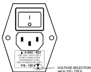
The correct values are given on the rear panel for the different line sources.
