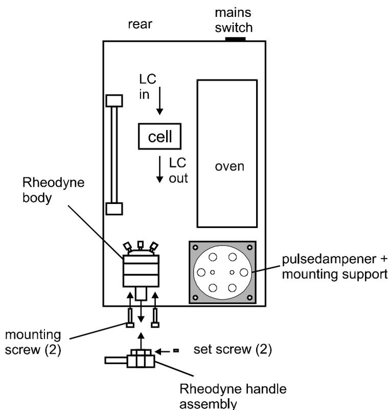
Fig. 2. Installation of the DECADE.
