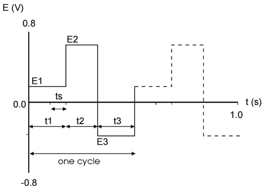
Fig. 18. Potential steps in pulsed amperometric detection. A part of  $t_1$  is used for detection ( $t_s$ ). The metal oxide layer that is formed during  $t_2$ , is removed during  $t_3$ , resulting in a renewal of the electrode surface.
