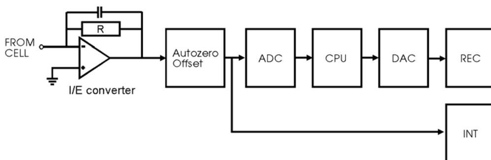
Fig. 4. DECADE signal processing from electrochemical flow cell to REC and INT output.  $R$  is a selectable resistor of 100, 10 or 0.1 MOhm corresponding to the pA, nA and  $\mu\text{A}$  range respectively.
