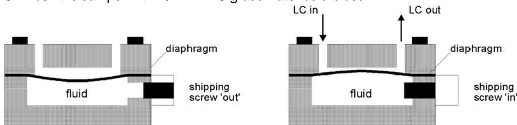
The shipping screw on the SSI pulse damper part no. 12-0125 must be firmly tightened (turn clockwise) before operating, or damage to the unit will result. The SSI pulse damper part no. 12-0625 is ready for use as supplied.
