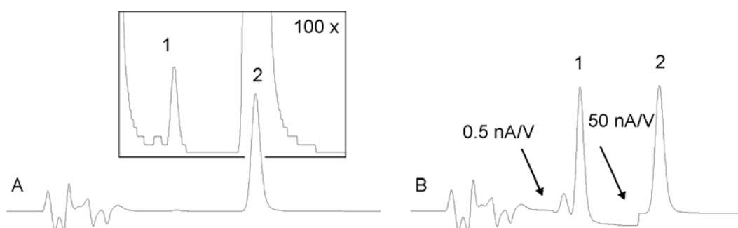
Fig. 10. Example of range programming to maintain the recorder resolution. In chromatogram (A) a range setting of 50 nA/V is used, in chromatogram (B) the output range is automatically switched during the run resulting in a considerable improvement of the output resolution of peak 1.
