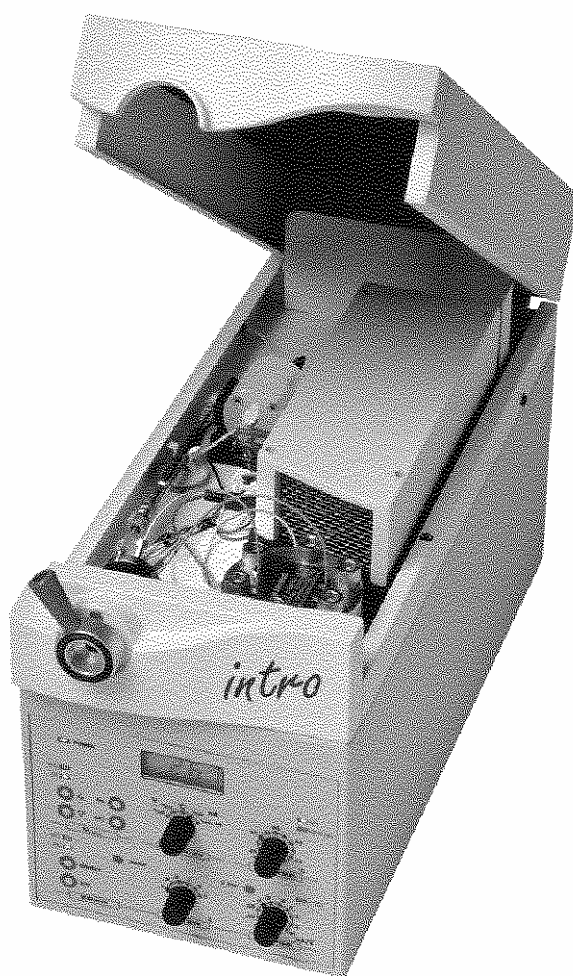
Fig. 1. The INTRO with Faraday-shielded oven compartment which accommodates flow cell, column, injector and pulse dampener.
