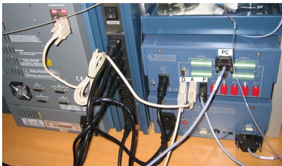
Fig. 31. Connectors AS 100, D - A - P order: d etector, a utosampler and p ump.
