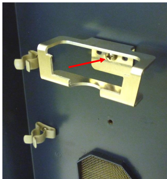
Fig. 6. \mu -PrepCell holder mounted on the centre position in the ROXY potentiostat oven compartment.
