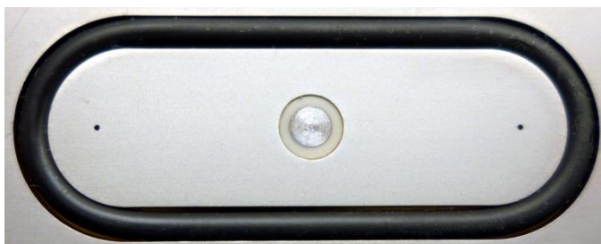
Fig. 9. The Reference electrode (centre) properly mounted in the inlet block.
