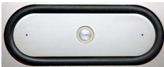
Fig. 15. The Titanium inlet block with Viton-O-ring.
