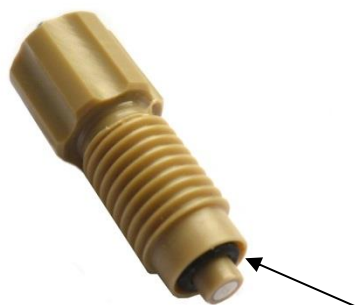
Fig. 8. Reference electrode with Viton O-ring (black arrow).
