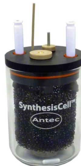
Figure 1. Synthesis Cell with Reticulated Glassy Carbon WE electrode (RGC).
