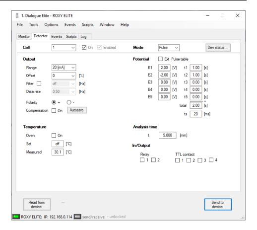
Set the parameters in the cell control window. It is recommended to set the Output Range to 20 mA. Set t3..5 to 0 s.
