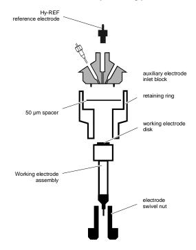
Fig. 6. Exploded diagram of ReactorCell.
