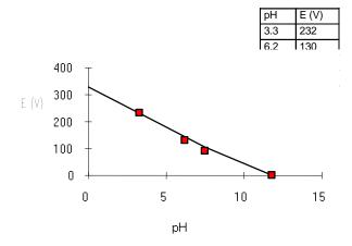
Fig. 3. Potential difference between HyREF and Ag/AgCl REF versus pH.
