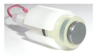
Fig. 9. Working electrode assembly with Magic Diamond electrode .
