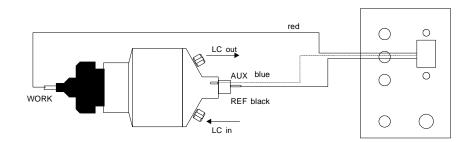
Fig. 5. ReactorCell and cell cable (for ROXY potentiostat<sup>™</sup>). WORK, AUX and REF are connected using the red, blue and black lead of the cell cable, respectively.
