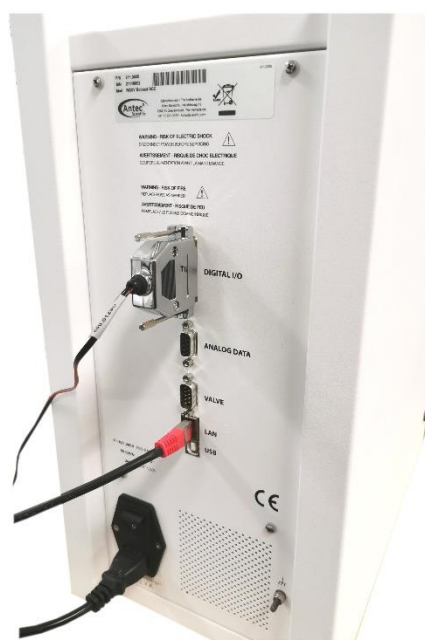
Fig. 3. Example of connections in the rear panel of the ROXY Exceed.
