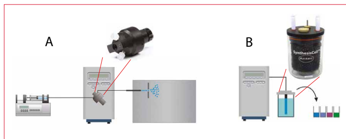
Figure 1: Schematics instrumental setup: (A) On-Line EC-MS for metabolite (transformation product, TP) generation using the ReactorCell. (B) Off-line EC-MS for metabolite (TP) synthesis using the SynthesisCell
