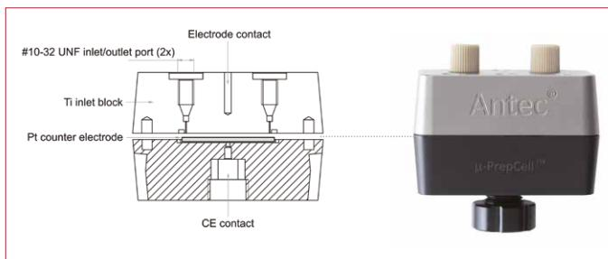
**Figure 2:** Figure 2: Dual electrode  $\mu$ -PrepCell SS consisting of a Titanium inlet block and a Platinum counter electrode.
