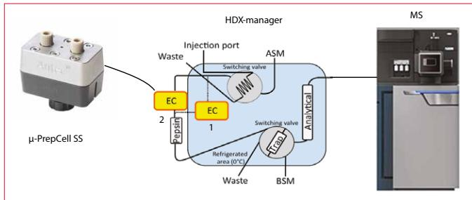
**Figure 1:** Schematics of a Waters HDX-MS (Synapt G2Si) system with an integrated  $\mu$ -PrepCell SS, controlled by a ROXY™ potentiostat with Dialogue Elite software. The electrochemical cell can be placed inside the HDX manager at 0°C (1) or outside at room temperature (2).
