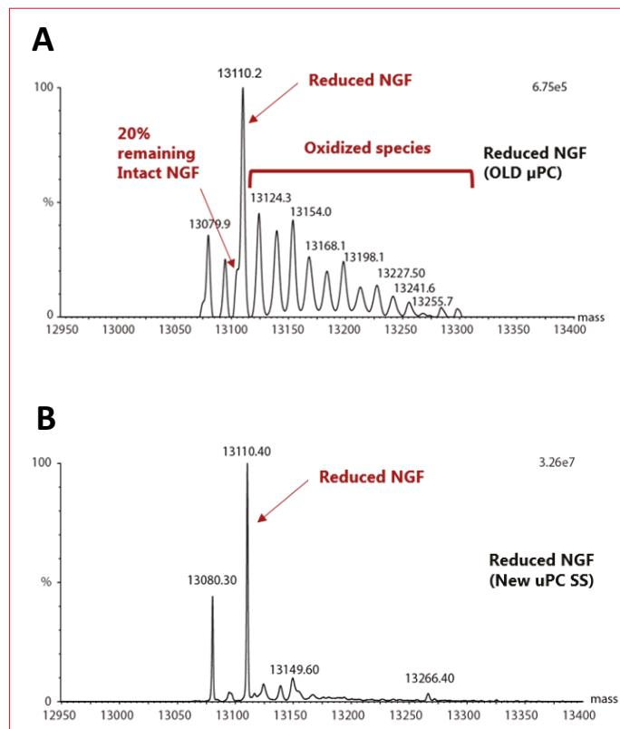
**Figure 4:** Comparison of mass spectrum of reduced Nerve Growth Factor (NGF) using a previous model of the  $\mu$ -PrepCell (A) and the new  $\mu$ -PrepCell SS (B).
