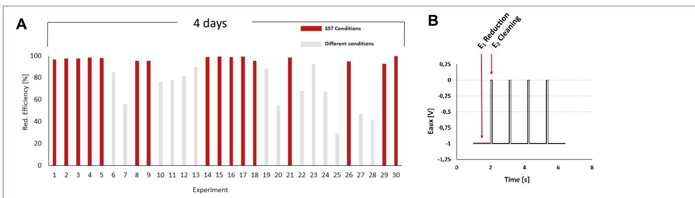
**Figure 3:** (A) Overview of the reduction efficiency of 10 pmol Bovine Insulin in a EC-HDX-MS set-up under SST (50 $\mu$ L/min and 1% FA at room temperature) and different conditions. (B) Standard pulse settings for disulfide bond reduction (E<sub>1</sub>, E<sub>2</sub>, t<sub>1</sub>,t<sub>2</sub>; 1.0V, 0.0V, 1.0s, 0.1s.). See next page for details about the experiments.
