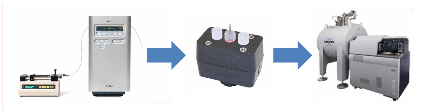
Figure 1: ROXY EC system equipped with the \mu -PrepCell2.0 and a proprietary Ti-Blue electrode was coupled with a Bruker SolariX 12T FT-ICR Mass Spectrometer for accurate protein MS and MS/Ms analysis
