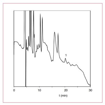
**Figure 3:** Chromatogram of purified and hydrolyzed lymphocyte DNA of a non-smoking volunteer. Peak 1 is 4 nmol/l (40 fmol) 8-OH-dGuo. Injection volume: 10  $\mu$ L. Condition see Table 3. Courtesy: ref [4]
