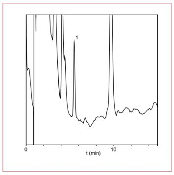
Figure 4: Chromatogram of purified and hydrolyzed rat spleen DNA treated with methylating agent. Peak 1 is 21 nmol/l (105 fmol) 7-MetGu. Injection volume: 5  $\mu$ L. Conditions see Table 4. Courtesy: ref [4]
