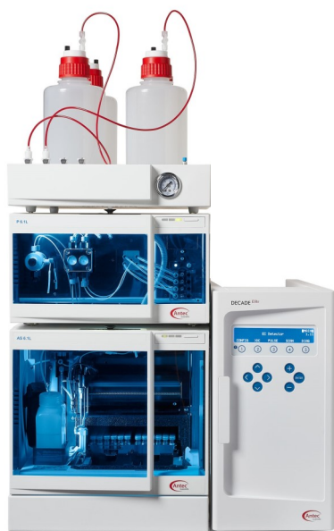
Figure 6: Recommended instrument configuration for this application: the ALEXYS HPAEC-PAD Analyzer The system consists of a P6.1L pump with integrated Solvent Switch Valve (SSV) capable of running step gradients, an AS6.1L autosampler, an ET 210 Eluent tray for helium blanketing, the optional CT 2.1 column oven with broadened temperature range, and the DECADE Elite electrochemical detector. The ALEXYS HPAEC-PAD Analyzer can be operated under different Chromatography Data System (CDS) software, namely DataApex™ Clarity™ CDS (version 8.3 and up) or Thermo Scientific™ Chromeleon™ CDS (version 7.2 SR 5 and up).
