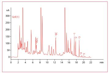
**Figure 11:** Chromatogram of 10x diluted and filtered wine (Santa Digna cabernet sauvignon 2003, Chile - sample '1'). Peaks: 1= myricetin, 2= transresveratrol, 3= quercetin, 4= cis-resveratrol and 5= kaempferol.
