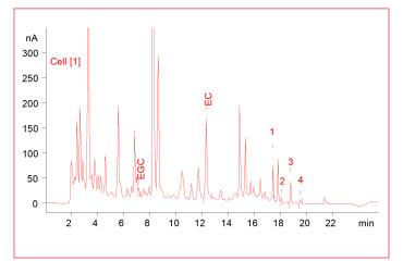
**Figure 13:** Chromatogram of 10x diluted and filtered wine (Vin de Pays d'Oc, vintage unknown, France - sample '3'). Peaks: 1= myricetin, 2= trans-resveratrol, 3= quercetin, 4= cis-resveratrol and 5= kaempferol.
