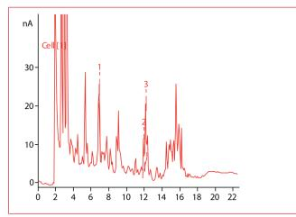
**Figure 7:** Chromatogram of 10x diluted and filtered hot black tea (bag of ca. 2 g Zonnatura black tea seeped for 5 min in 0.2 L hot water). Peaks: 1= EGC, 2= EC and 3= EGCG.
