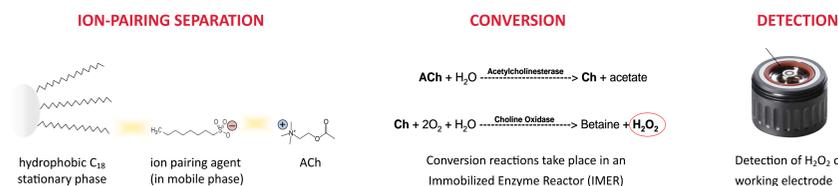
Fig. 3 Principle of acetylcholine analysis. The analysis of acetylcholine is based on ion-pairing separation, followed by an enzymatic conversion and electrochemical detection of hydrogen peroxide on a platinum working electrode.
