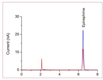
Figure 4: Chromatogram of (1) Blue curve: 0.01% Epinephrine sample pH 4, diluted 40x (2.5 ppm). Red curve: 0.01% Epinephrine sample pH 8-9, diluted 40x (2.5 ppm). Injection volume 2  $\mu$ L.
