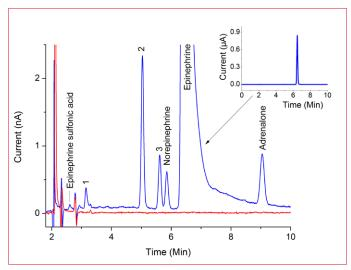
**Figure 6:** Blue curve: zoom-in on baseline of the chromatogram of the undilut-ed 0.01% Epinephrine sample pH 4. Top-right insert: full chromatogram. Red curve: blank injection of diluent. Injection volume 2  $\mu$ L.
