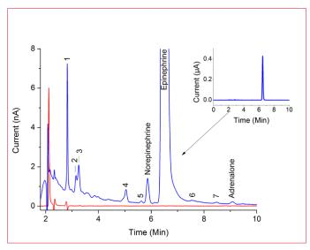
**Figure 7:** Blue curve: zoom-in on baseline of the chromatogram of the undilut-ed 0.01% Epinephrine sample pH 8-9. Top-right insert: full chromatogram. Red curve: blank injection of diluent. Injection volume 2  $\mu$ L.
