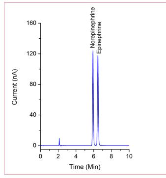
**Figure 1:** 2  $\mu$ L injection of a 22  $\mu$ g/mL Epinephrine Bitartrate RS and 20  $\mu$ g/mL Norepinephrine Bitartrate RS solution in 0.5 mg/mL Potassium Metabisulfite (System suitability solution as described in the USP monograph).
