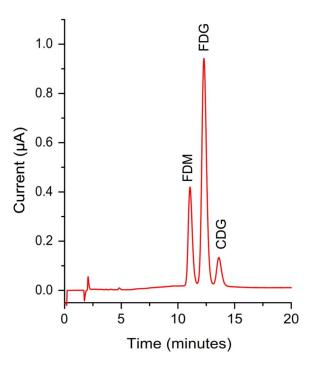
Fig. 1. Chromatogram obtained with a 10  $\mu$ L injection of a 50  $\mu$ g/mL CDG, FDG and FDM standard mixture in water .
