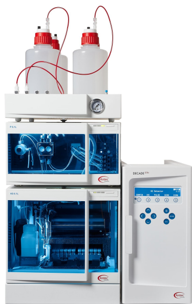
Figure 5. Recommended instrument configuration for this application: the ALEXYS Carbohydrate Analyzer The system consists of a P6.1L pump with integrated Solvent Switch Valve (SSV) capable of running step gradients, an AS6.1L autosampler, an ET 210 Eluent tray for helium blanketing, and the DECADE Elite electrochemical detector. A CT 2.1 column oven with broad temperature range can be added optionally. The ALEXYS Carbohydrate Analyzer can be fully controlled by different Chromatography Data System (CDS) software, namely DataApex™ Clarity™ CDS (version 8.3 and up) or Thermo Scientific™ Chromeleon™ CDS (version 7.2 SR 5 and up).
