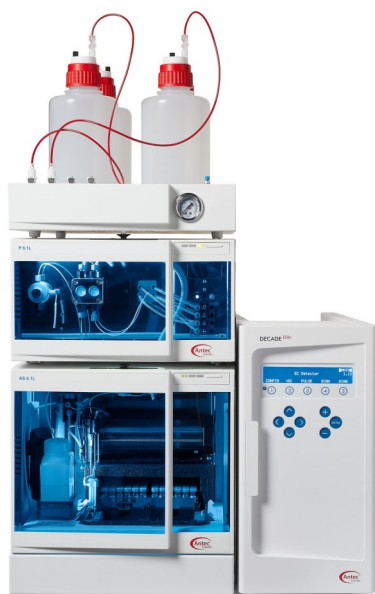
Figure 6: The ALEXYS analyzer for Erythromycin, consisting of the ALEXYS Antibiotics base system - Gradient, and dedicated flow cell and bottles. The base system consists of a LPG quaternary gradient P6.1L pump with integrated degasser, an AS6.1L autosampler, an ET 210 Eluent tray for helium blanketing, and the DECADE Elite electrochemical detector. The system is delivered with DataApex™ Clarity™ Chromatography Data System (CDS) software. Optionally, control drivers are available to operate the system in Thermo Scientific™ Chromeleon™ CDS (version 7.2 SR 5 and up).
