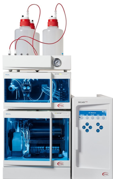
Figure 5: The ALEXYS analyzer for Streptomycin, consisting of the ALEXYS Antibiotics base system - Isocratic, and dedicated flow cell and bottles. The base system consists of a P6.1L pump with integrated Solvent Switch Valve (SSV) capable of running step gradients, an AS6.1L autosampler, an ET 210 Eluent tray for helium blanketing, and the DECADE Elite electrochemical detector. The system is delivered with DataApex™ Clarity™ Chromatography Data System (CDS) software.
