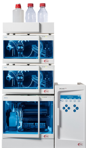
Figure 9. The ALEXYS analyzer for Spectinomycin and Lincomycin, consisting of the ALEXYS Antibiotics base system - isocratic, post-column addition kit (NaOH) and FlexCell with gold working electrode, HyREF and stainless steel auxiliary electrode. The ALEXYS analyzer is fully controlled by DataApex™ Clarity™ software.
