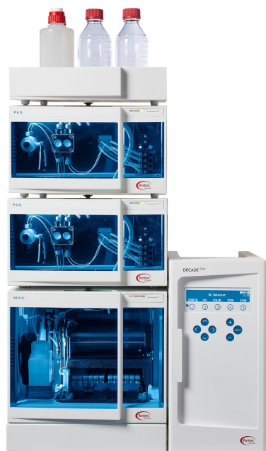
Figure 2. The ALEXYS analyzer for Gentamicin, consisting of the ALEXYS Antibiotics base system - isocratic, post-column addition kit (NaOH) and FlexCell with gold working electrode, HyREF and stainless steel auxiliary electrode. The ALEXYS analyzer is controlled by DataApex™ Clarity™ software.
