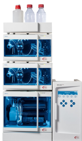
Figure 1: ALEXYS analyzer for analysis of Netilmicin.
