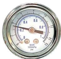
Flow regulator valve with pressure gauge displaying the actual He pressure in psi and bar
